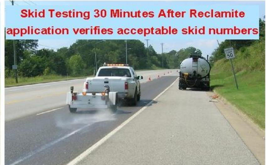
Skid Testing 30 Minutes After Reclamite application verifies acceptable skid numbers
